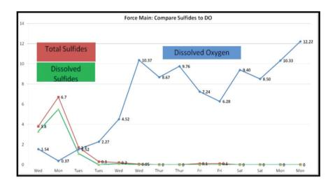
Anue's oxygen delivery technology provides beneficial O2 to the force main, creating a positive dissolved Oxygen level eliminating the corrosive anaerobic SRB activity there by reducing costly maintenance and repair while extending life in collection systems.
